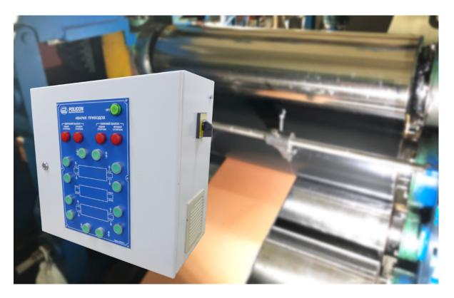
The modernization of the calender includes the installation of a new automation cabinet with a control panel.
